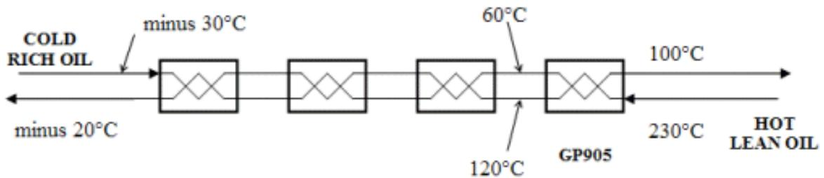
*Fig. 1 – Extremely simplified schematic arrangement of GP905 & other exchangers (temperatures are nominal only, for normal operations)*
